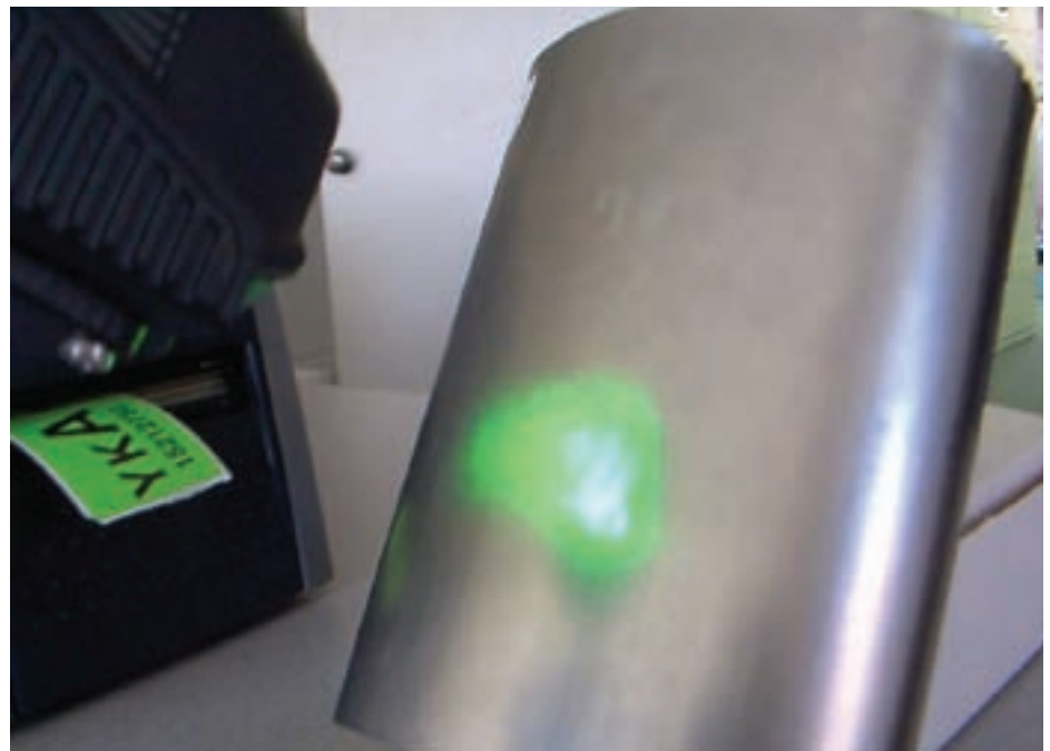
When the scanner successfully reads the Eberspächer part mark, a customer part label is printed.
